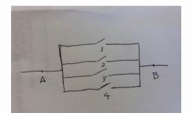
A system composed of *n* separate components is said to be a parallel system if it functions when at least one of the components functions. For such a system, if components *i*, independent of all other components, functions with probability  $p_i$ , then the probability that the system functions is
